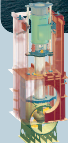
"Libas" was the first trawler/purse-seiner in the world, equipped with a Combined Retractable Azimuth Tunnel Thruster. Brunvoll AR 80, 1470kW
