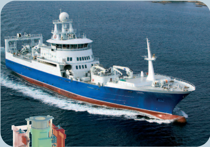
"Libas" was the first trawler/purse-seiner in the world, equipped with a Combined Retractable Azimuth Tunnel Thruster. Brunvoll AR 80, 1470kW
