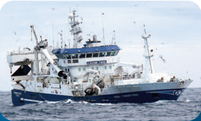
"Finnur Fridi" – trawler/purse-seiner built at Aker Langsten AS (STX) for Krossbrekka PF, Færøylene. 2x Brunvoll 882 kW tunnel thruster bow/stern.
