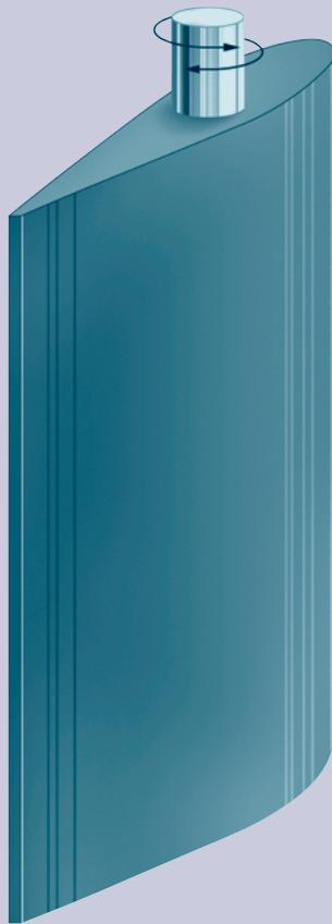
The Van der Velden® ATLANTIC rudder has no moving parts, which significantly increases its life-span. The profile design and rudder shape can be adapted to suit specific vessel requirements. Examples include minimising drag and cavitation danger for high-speed vessels, or reducing noise and vibration levels for comfort.
